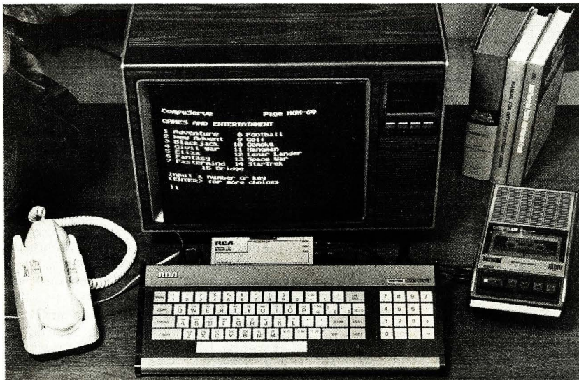
The RCA VP3501 Videotex Data Terminal has r-f modulator and modem.
