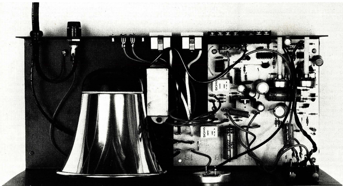
Inside view of pre-entry detector component layout based on author's pc board layout.
